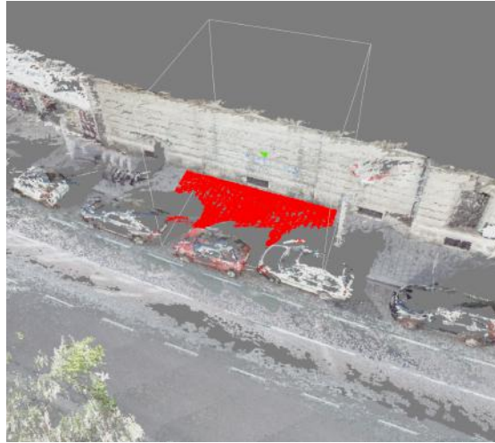
Figure 3.2: Point cloud where the floor was successfully detected. Points marked red = inliers.
