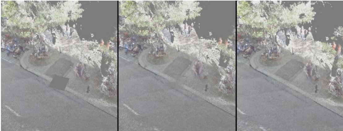
Figure 4.23: Point cloud that has been image inpainted. On the right side, the ground truth is visible.
