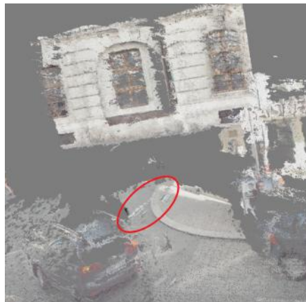
Figure 4.9: Outlier points of the wall are highlighted with a red circle.
