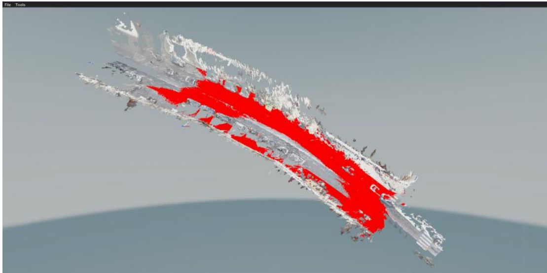
Figure 3.3: Point cloud where the ground is not fully recognized. Points marked red = inliers, the grey area interior to the red area should also be marked.
