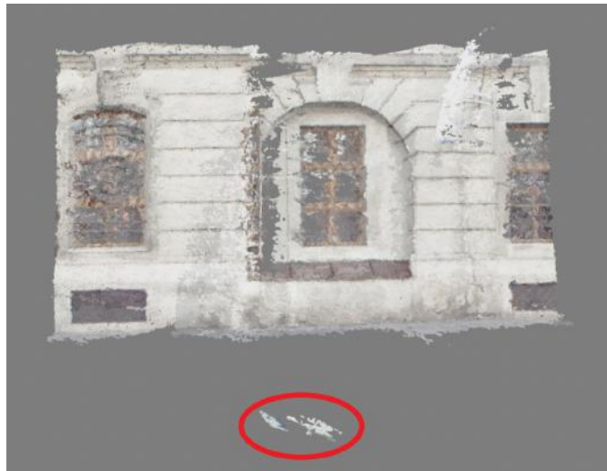
Figure 4.7: Wall with outliers below the lowest point of the wall. Outliers are highlighted with a red circle.
