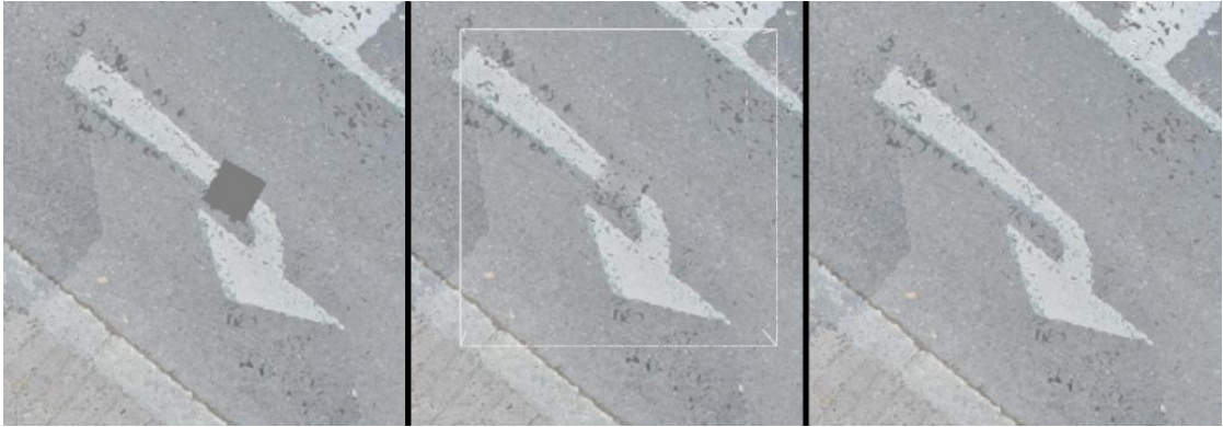
Figure 4.24: Point cloud that has been image inpainted. On the right side, the ground truth is visible.
