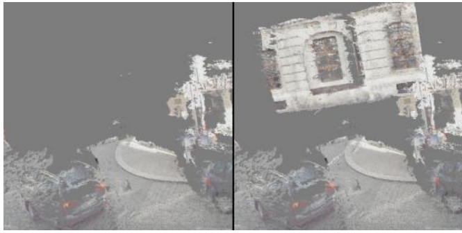
Figure 4.8: The addition of a wall to a scene (right image). The wall is not on the ground as would be desired.
