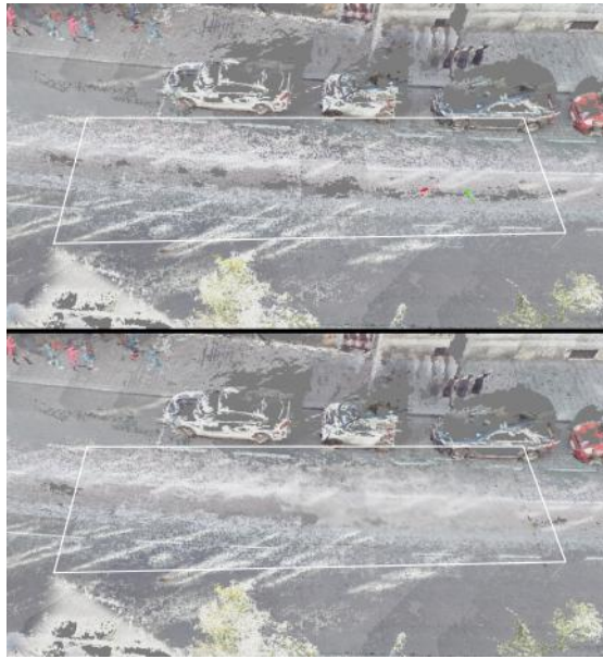
Figure 4.13: Image inpainting on a selected area of approximately 100,000 points.
